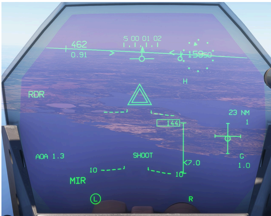
Target tracked by the radar and missile seeker, with the left MICA IR ready to fire
