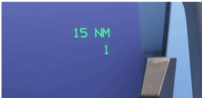
Primary goal number 1 and its distance displayed on the HUD
