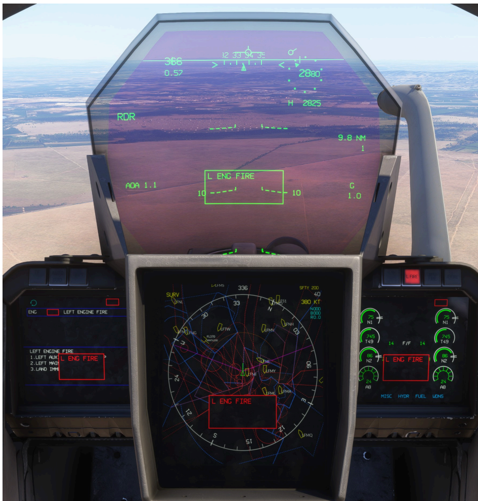
Red alarm displayed on main avionics screens
