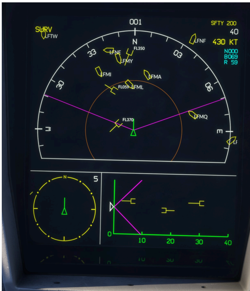
Center display showing three detected aircraft
