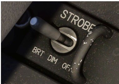
Strobe lights switch
