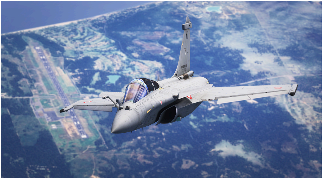
View showing the delta wings and canards
