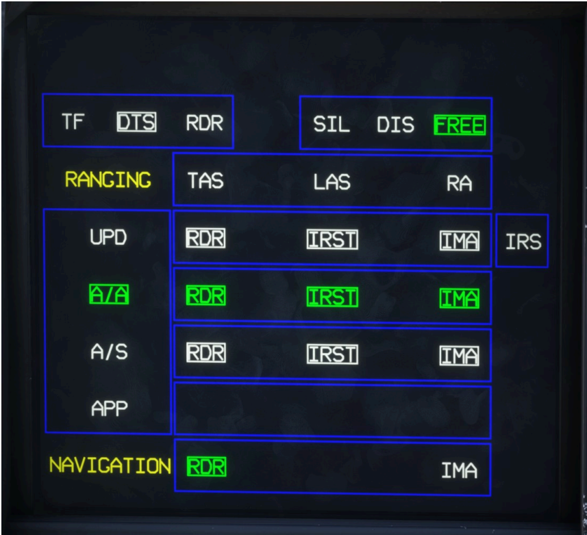
LD SYS page with radar selected and active in A/A mode
