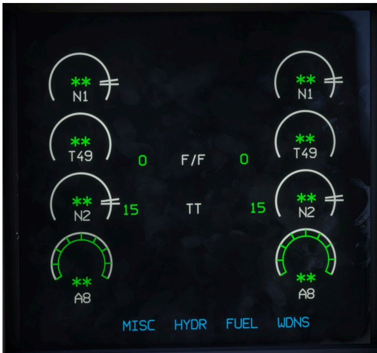
Display with the engine control units unpowered
